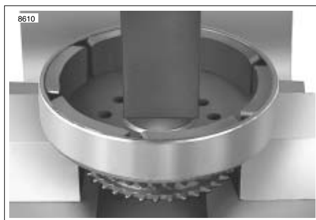
Figure 7-33. Removing Rotor From Sprocket
