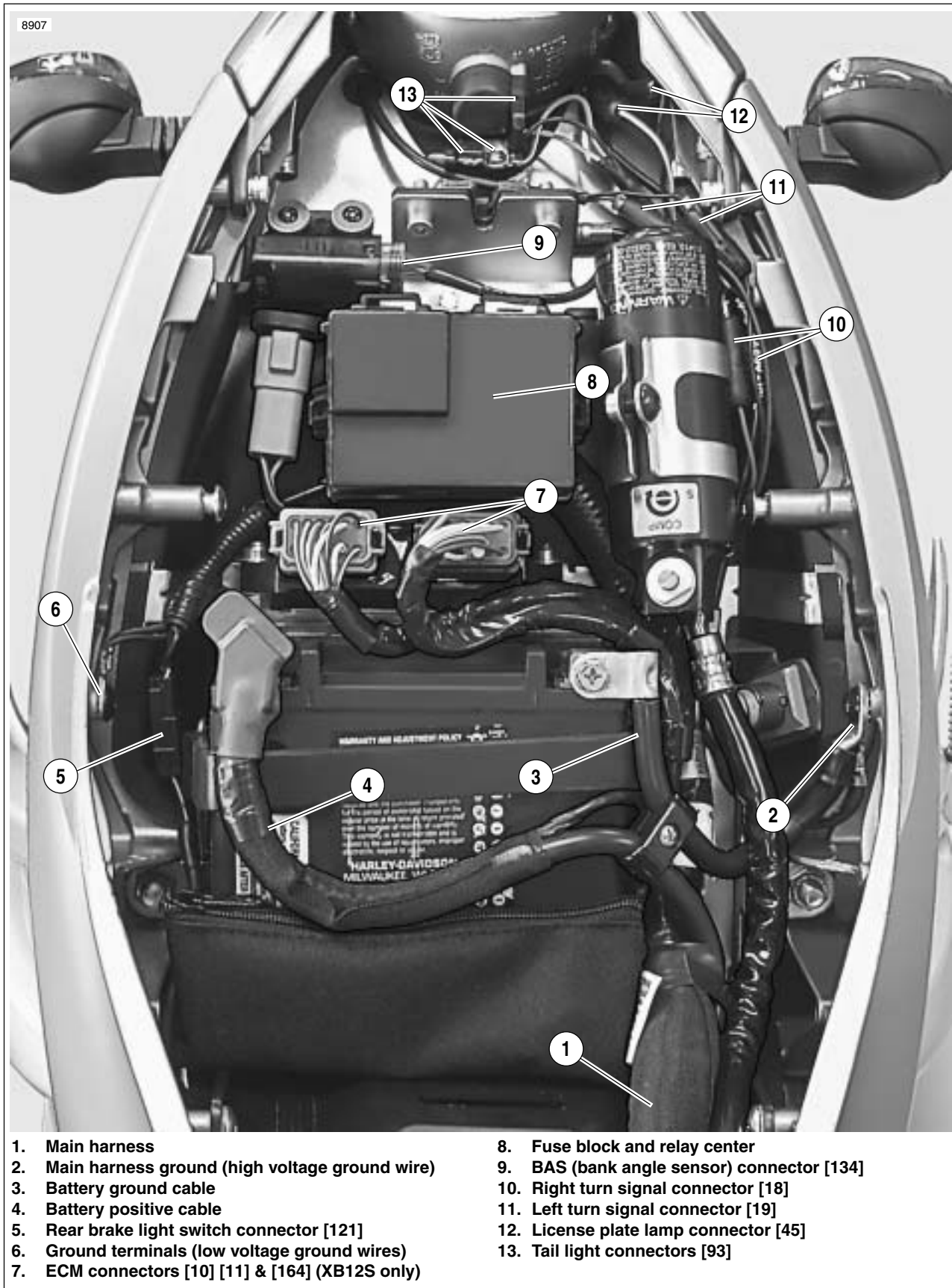
Figure 7-85. Main Harness and Electrical Connectors Under Seat
