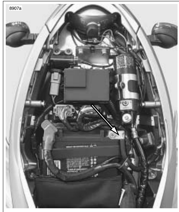
Figure 7-44. Negative Battery Cable
