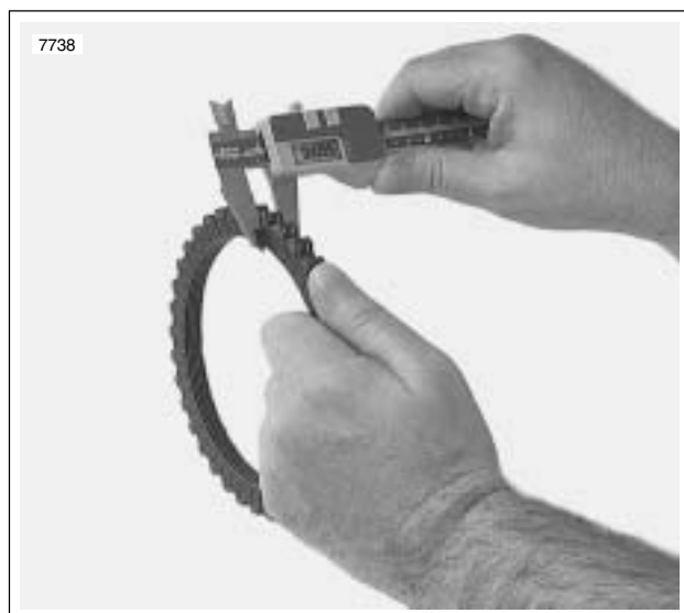
Figure 6-14. Measuring Friction Plates
