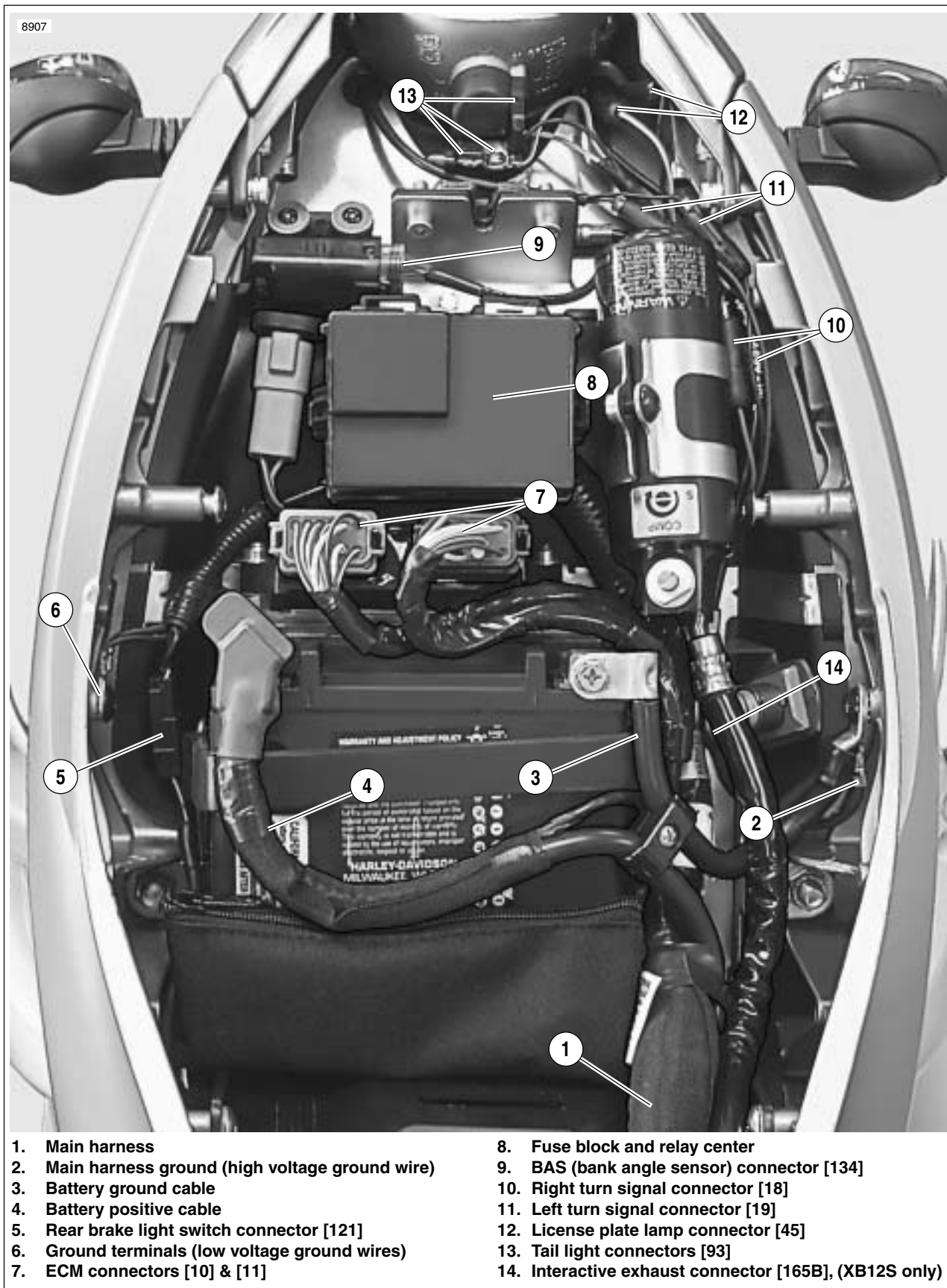
Figure 7-80. Main Harness and Electrical Connectors Under Seat
