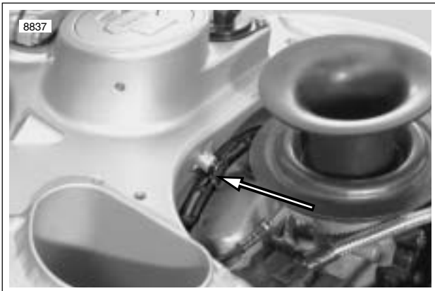
Figure 7-82. Wire Harness Clip
